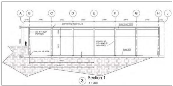
Figure 5. Detail showing sub-surface depth ( $\sim$  3.2m) to which the proposed construction will extend
